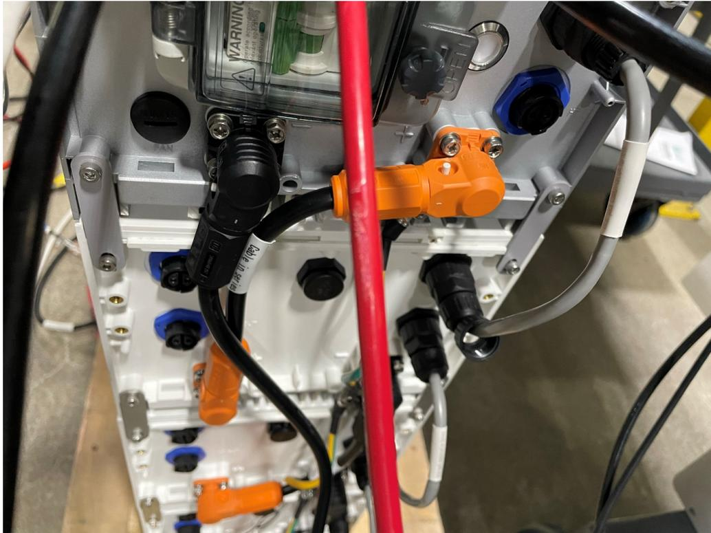
Utilize a multimeter to ensure the voltage between the positive (+) and negative (-) wires coming to the BMS.
